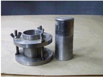
Figure 5. Reinforced crushing pot designed by Lőrincz [3]
