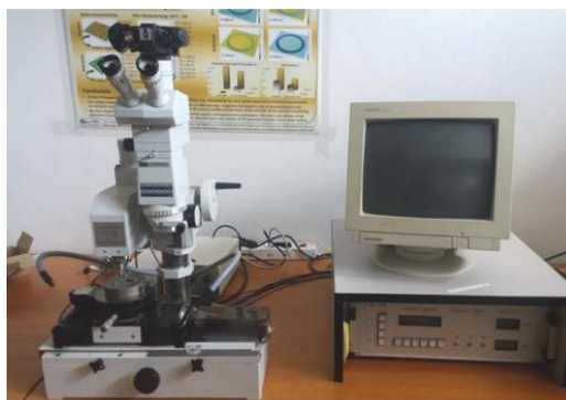
Figure 1. The SP-15 instrumented scratch tester
