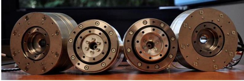
Figure 3. Prototypes of modular flat- and cylindrical wheel strain wave drive systems
