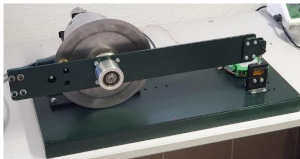
Figure 8. Test bench for the precision drive units
